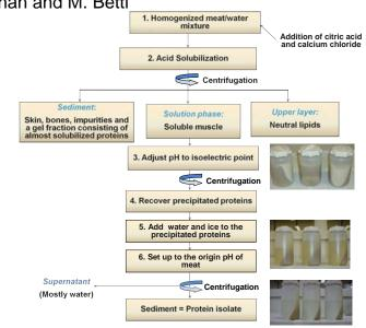
Figure 2. Schematic diagram of the protein extraction process
