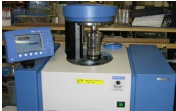
The calorimeter measuring energy values of feedstuffs & in vitro residues.
