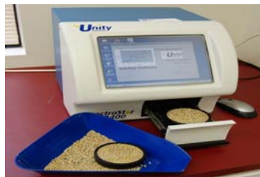
Feedstuffs are scanned by a calibrated NIRS machine.
