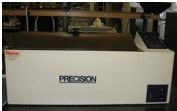
Shaking water bath mimicking body temperature & gut motility.
