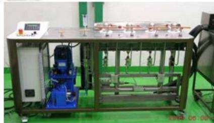
Figure 2. High Pressure Processing Machine (U111, UNIPRESS equipment division, Warsaw, Poland)
