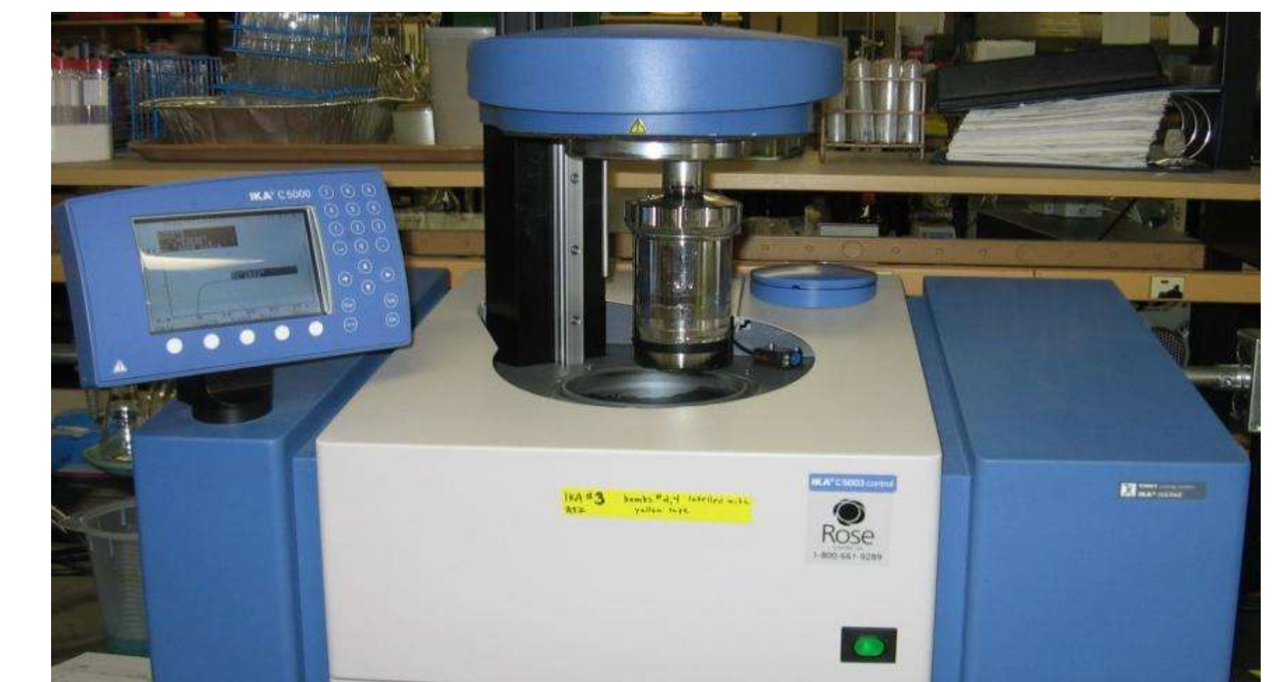
The calorimeter measuring energy values of feedstuffs & in vitro digestion residues.
