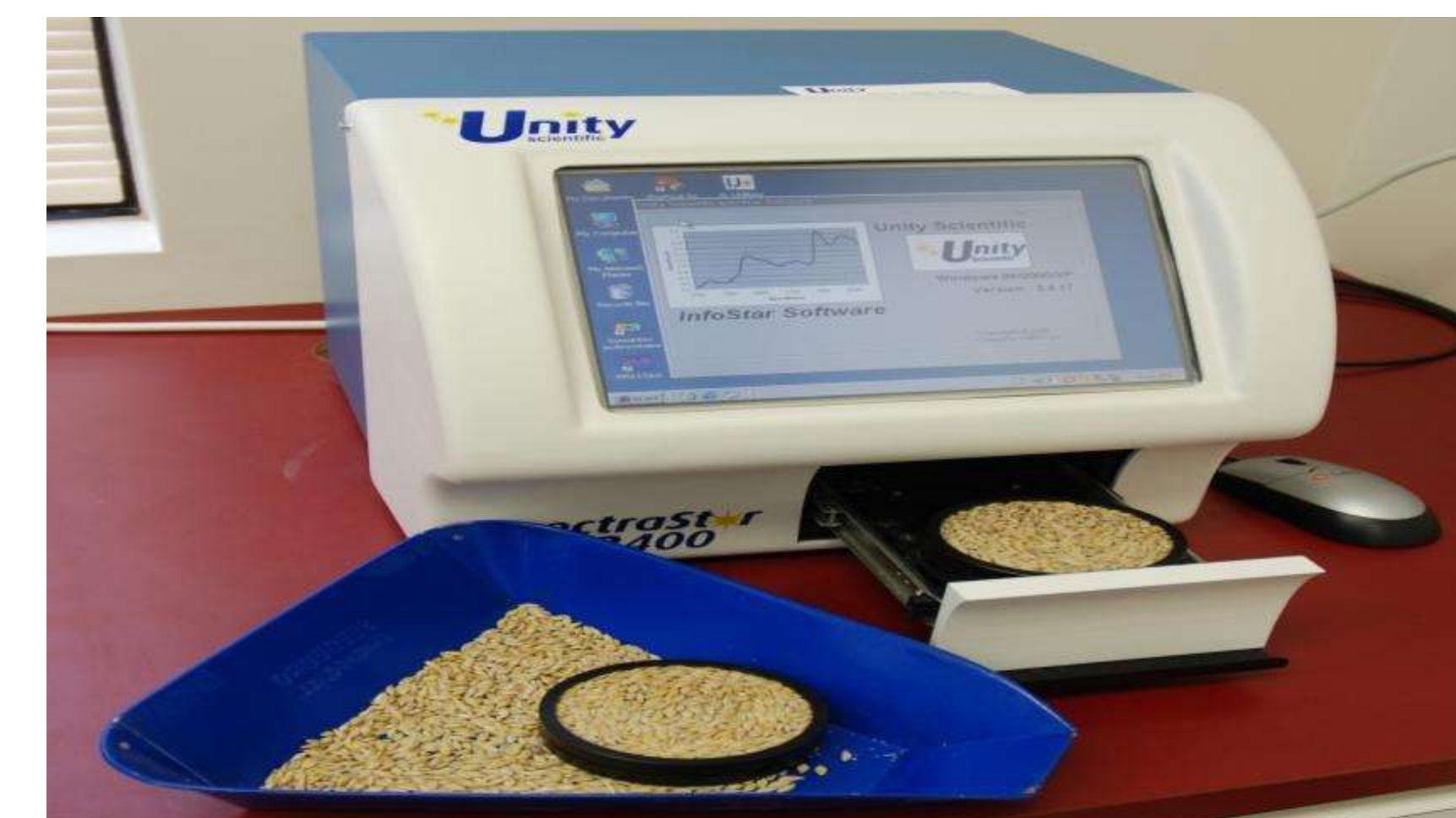
Feedstuffs are scanned by calibrated NIRS machine.
