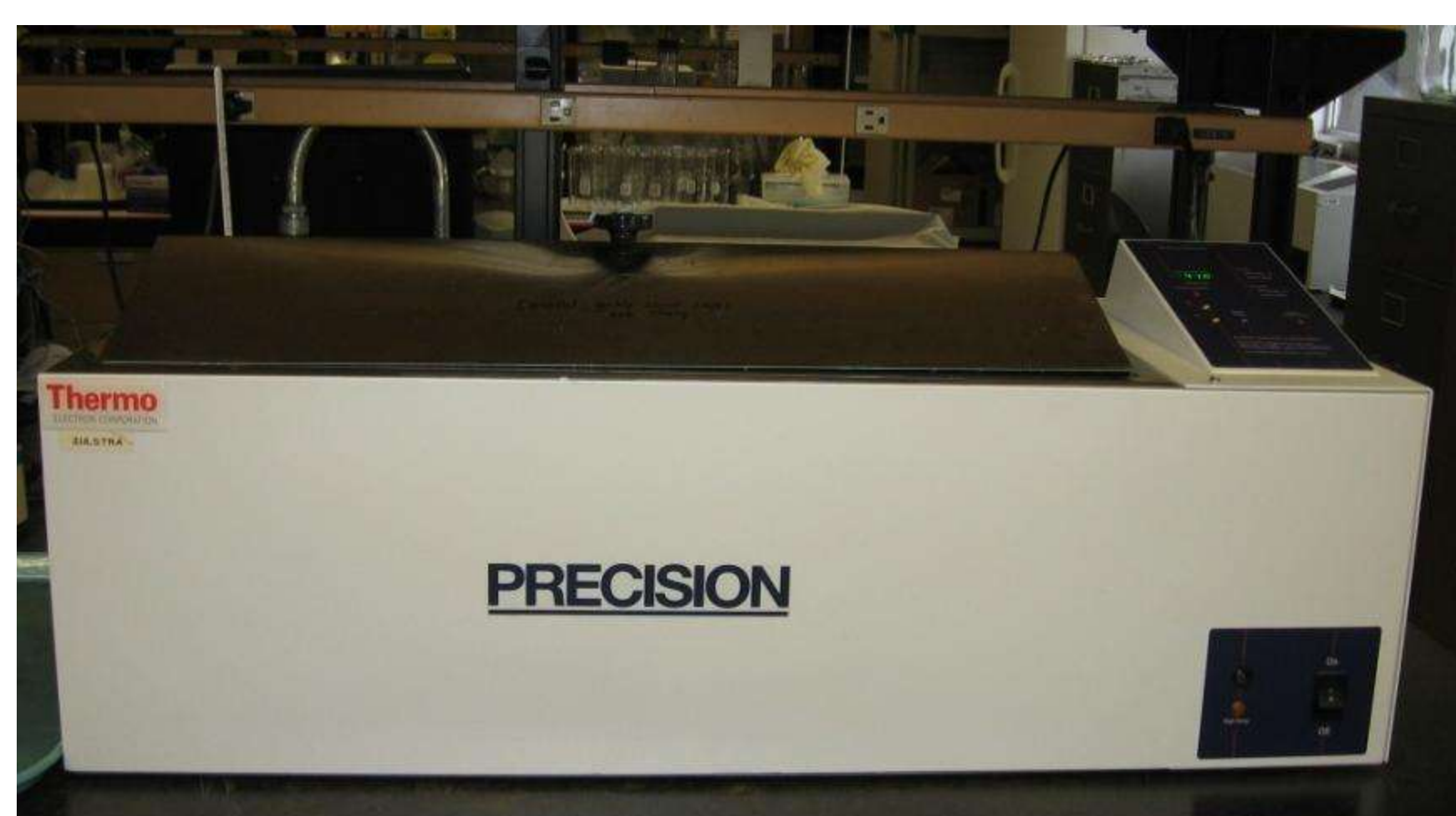
Shaking water bath mimicking body temperature & gut motility.
